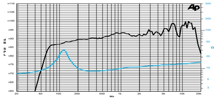
Frequency Response on 18 Lt @ 70 Hz Vented Box @ 1W, 1m
